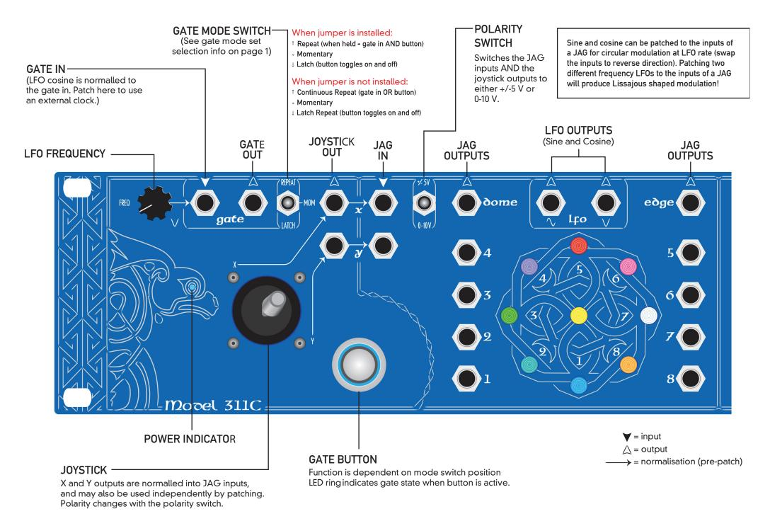
Allow a minimum case depth of 75mm behind the panel to allow clearance for the power connector when the cable is connected.
