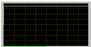
Waveform 15: A high DC offset.
